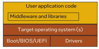
Target model includes all software-visible functional aspects of hardware, such as processor instructions, supervisor modes, device registers, interrupts, etc.
